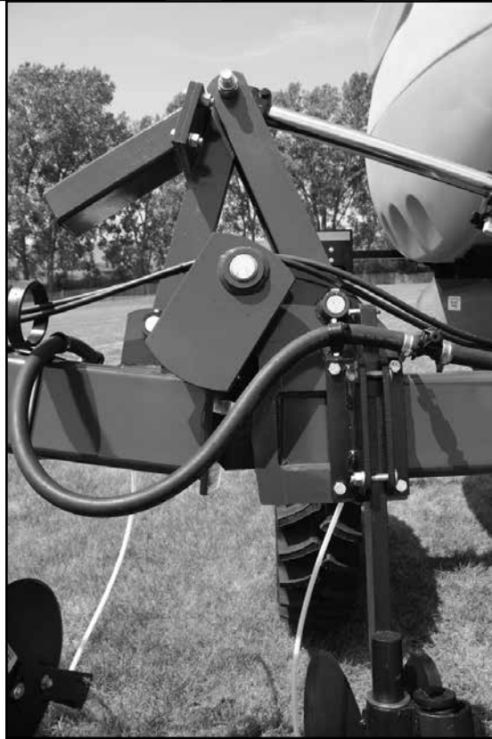
(Gull Wing hose 54") Primary wing hinge (30" row spacing)
